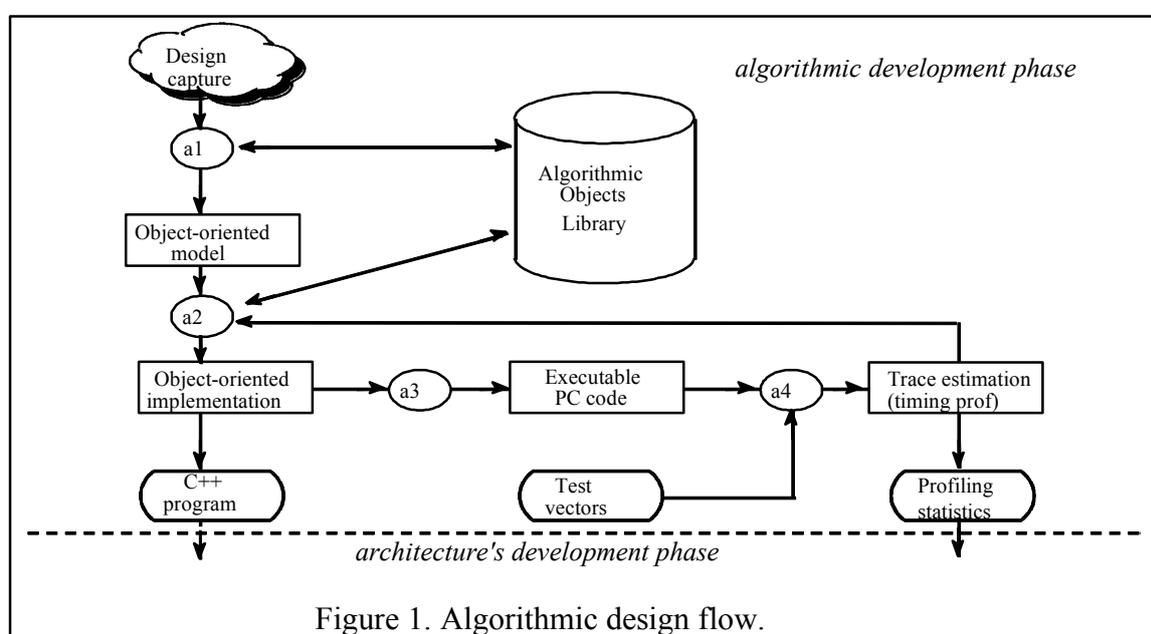
Figure 1. Algorithmic design flow.
