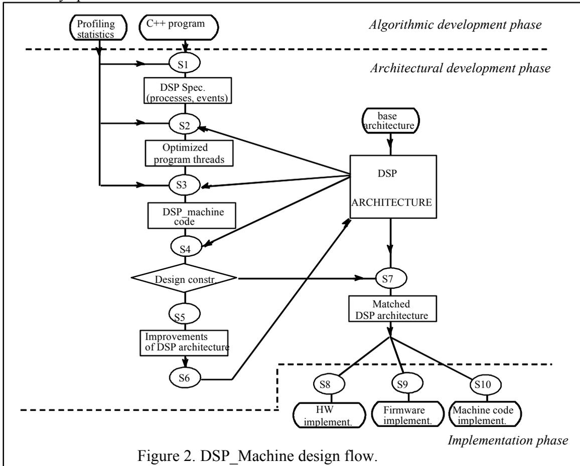
Figure 2. DSP\_Machine design flow.
