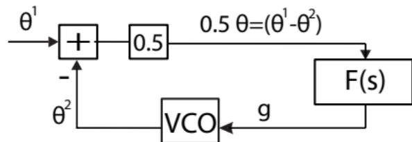
**Linearization:** while this is useful for studying loops that are near lock, it does not help for analyzing the loop when misphasing is large.
