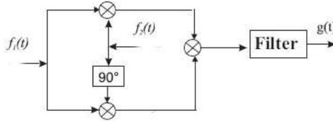
Figure 5: Three multipliers and filter
