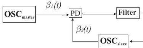
Figure 7: Block-diagram of PLL with squarer and the Costas loop
